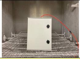
3. Test for protection against solid foreign 4. Test for protection against solid foreign objects (Dust test)
